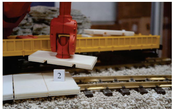
Figure 5 Robotic panel laying
