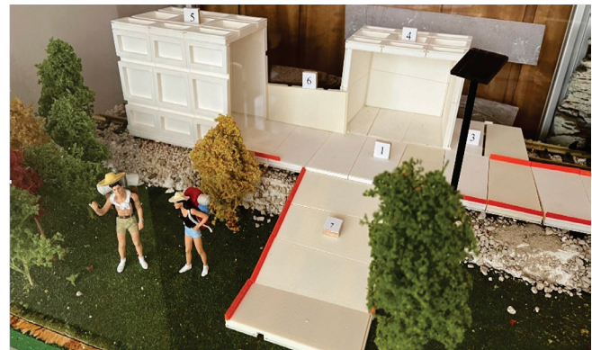
Figure 4 Mockup of provided options of the variable prefabricated panel system. Legend: 1 - covering of straight tracks, 2 - covering of curved tracks, 3 - covering of platforms, 4 - shelters, 5 - tunnels and underpasses, 6 - protection against landslides, 7 - easy bridging
