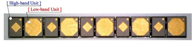
Figure 1 A 5G ceramic chip antenna array, displaying a module that combines a high-band unit and a low-band unit ceramic chip antenna, arranged in a 1 x 5 configuration.
