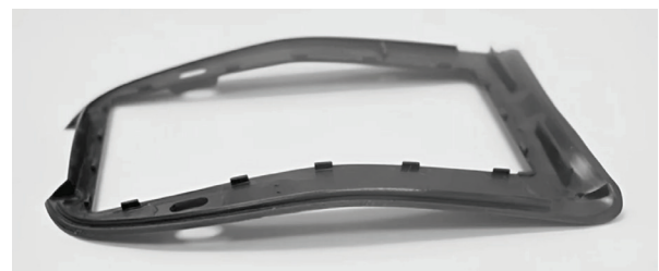
Figure 1 Example of moulded part warpage [1]
