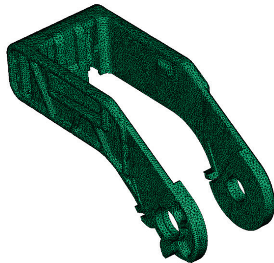
Figure 4 3D mesh model of a handle [6]
