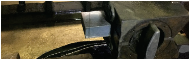
Figure 3 Cutting the sample on the wire EDM machine
