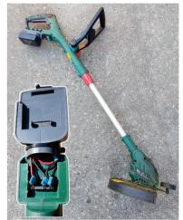
Figure 10 New trimmer with the old battery. Enlarged detail shows the wiring.
