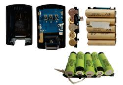
Figure 5 Repairment of the defective battery pack with a nominal capacity of 1.5 Ah with new cells with a capacity of 3.4 Ah.
