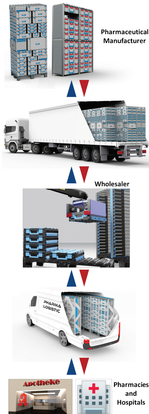
Figure 2 The vision of DigiPharmaLogNet. The RTI solution to be developed by the project team has a modularity mechanism incorporated, which allows stacking boxes with different sizes. Its compatibility with a robotic system enables automation of warehouse processes. Since RTIs are intended for reuse, circular logistic chains could be established in pharma logistics. RTI, returnable transport item.
