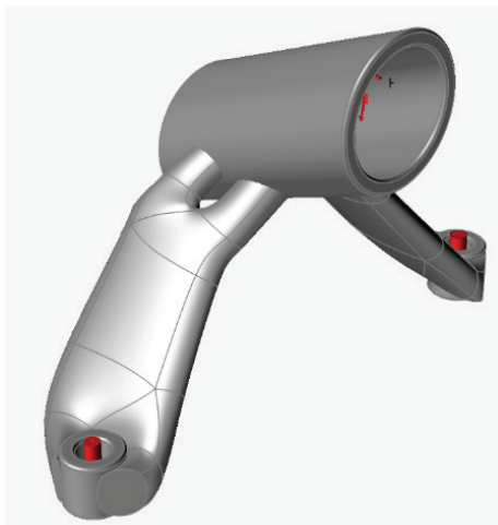
Figure 20 Post-processed topology optimized design (max. stiffness) [11]
