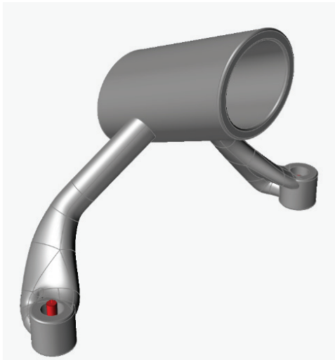
Figure 15 Post-processed topology optimized design (minimized mass) [11]
