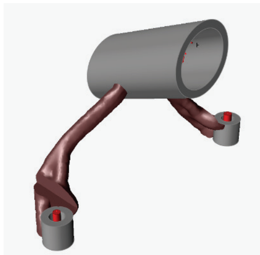
Figure 11 Topology optimized design – minimized mass [11]
