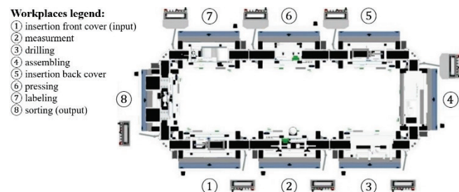
Figure 1 FESTO CP LAB 400 layout [26]
