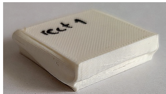
Figure 6 Compression specimen after the testing
