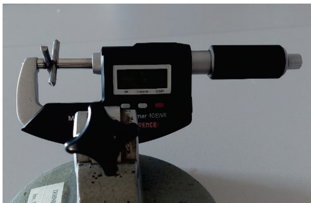
Figure 4 Measurement of setdown on samples using a digital micrometer
