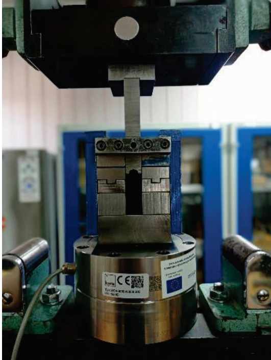
Figure 1 Cross-wire weld test setup
