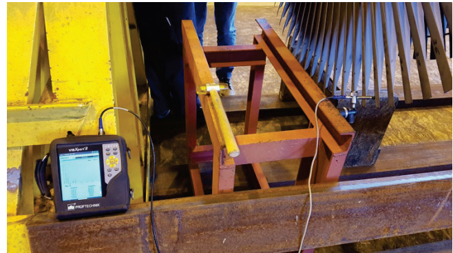
Figure 5 Measurement of natural frequencies of the rotor blade
