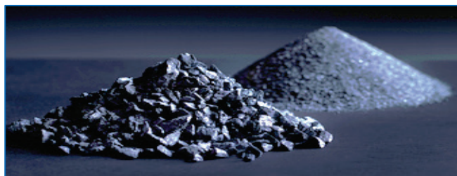
Figure 2 Silicon-based (light) pre-alloys used as nodulizer
