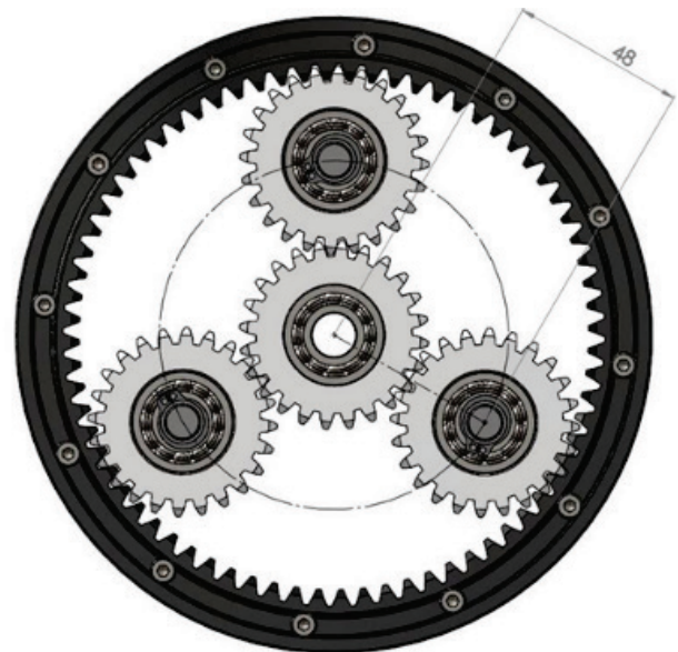
Figure 5 Inside gears of planetary gearbox
