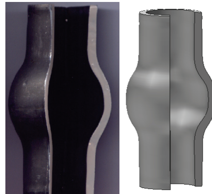
Figure 8 Properly deformed part obtained experimentally (left) and by numerical simulation (right)
