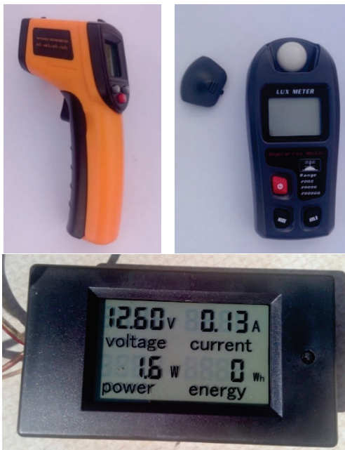
Figure 7 Lux meter Vktch mt30, Thermometer OUTEST GM320 and measuring Module Inpelanyu C01413
