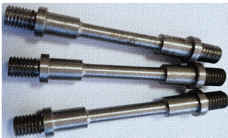
Figure 2 Austenitic stainless steel's sample for determining the hot deformability by torsion
