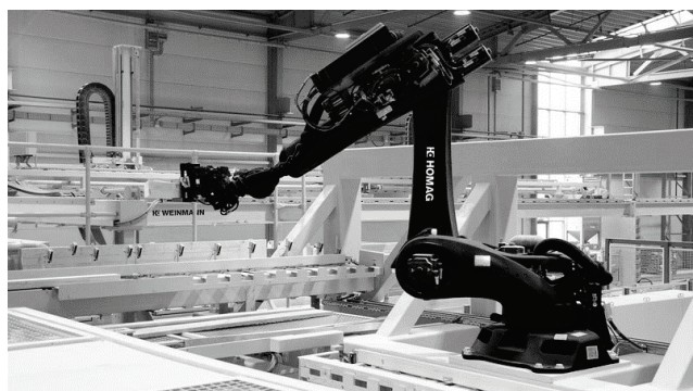
Figure 3 Robots used for manufacturing frame works in prefabricated housing construction [25].
