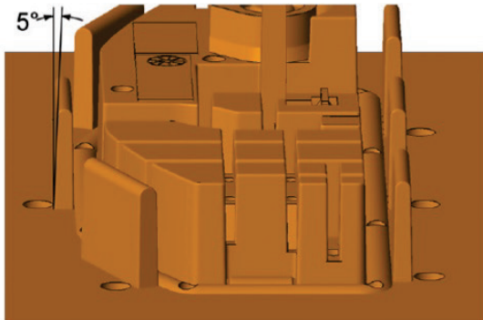
Figure 8 Increased draft angles [5]
