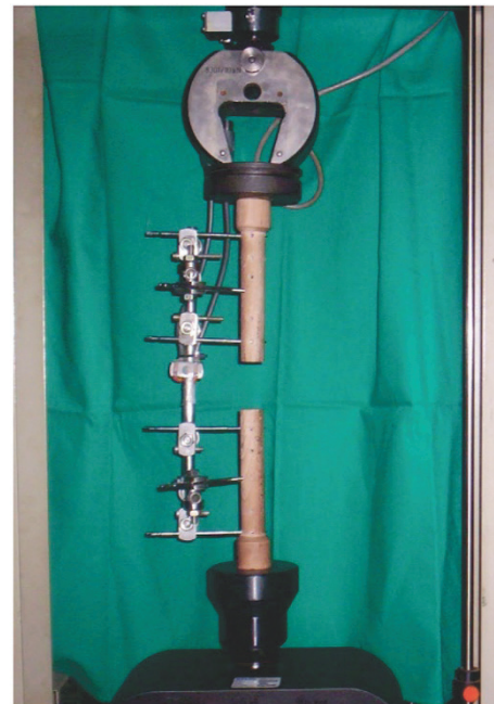
Figure 4 Fixator experimental setup
