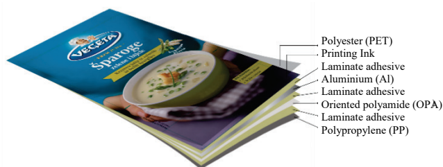
Figure 1 Multi-layered Stand-up Pouch Material
