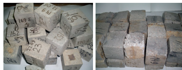
Figure 4 The material research: a) material samples prior to freezing and the thawing test; b) material samples after freezing and the thawing test (F 200)
