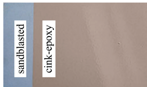
Figure 3 The view of the test sample: CINK-EPOXY primer
