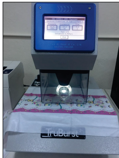
Figure 9 Bursting strength test (pneumatic method)
