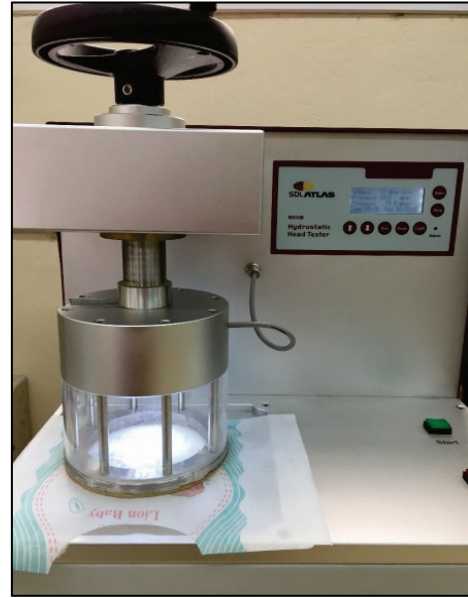
Figure 8 Water resistance test (dynamic test)
