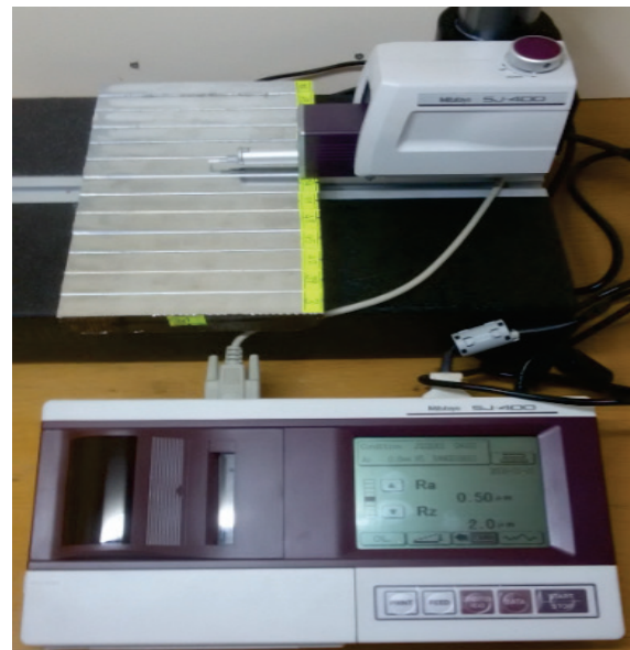
Figure 2 Surface roughness of the measurement device
