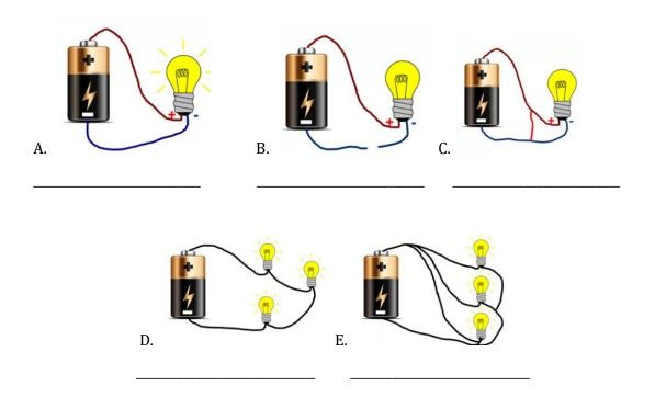
When two or more loads (Bulb, CFL, LED, Fan etc) are connected to each other in parallel, then it is called Parallel Circuit. In this type of circuit, the voltage capacity of all loads must be equal to input supply. The power of the "load" can be different. In a parallel circuit, if one load or bulb gets fused, then the rest of the bulbs will still get power supply and will glow.
