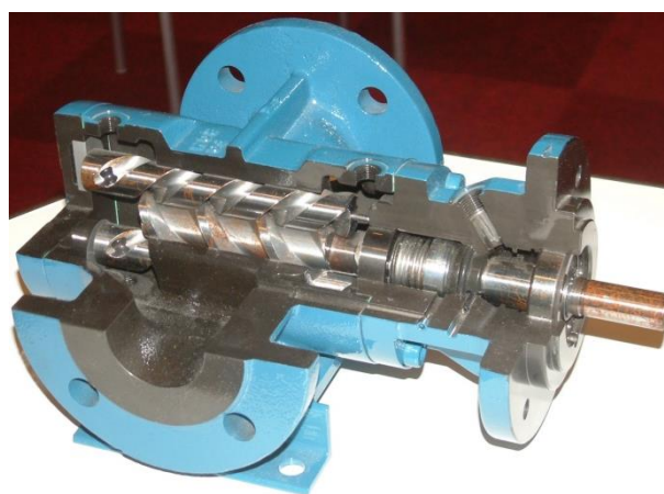
Figure 5. Cross-section of a horizontal construction of the three-spindle screw pump [5]
