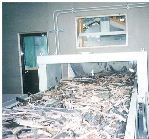
Figure 2. Example of a conveyor-belt for manual classification of materials [5]
