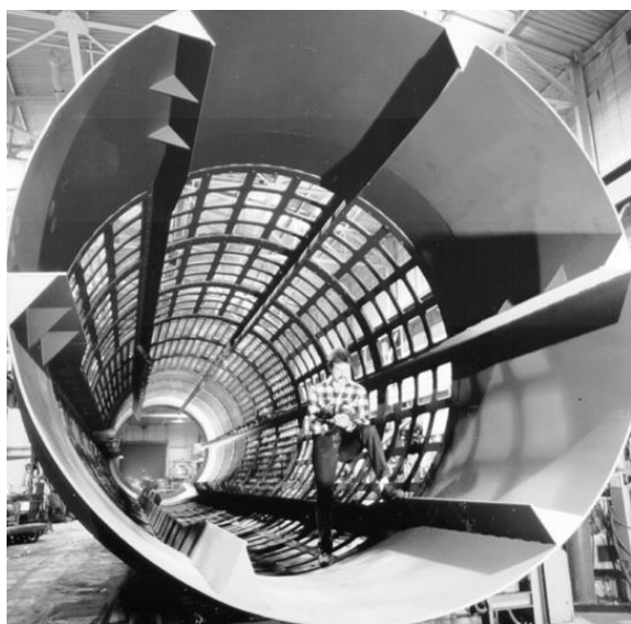
Figure 3. End view of a trommel screen [4]
