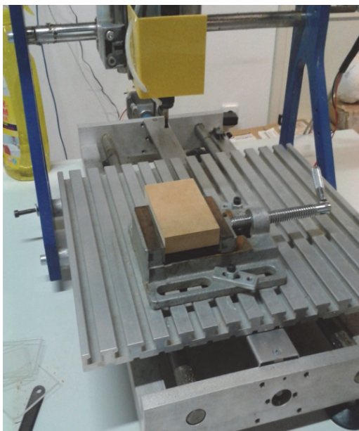
Figure 23 Block in place prepared to find the starting point (the 0 point) [5]
