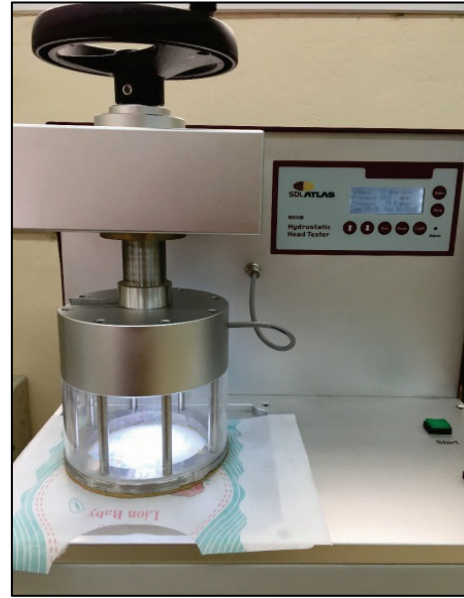
Figure 8 Water resistance test (dynamic test)
