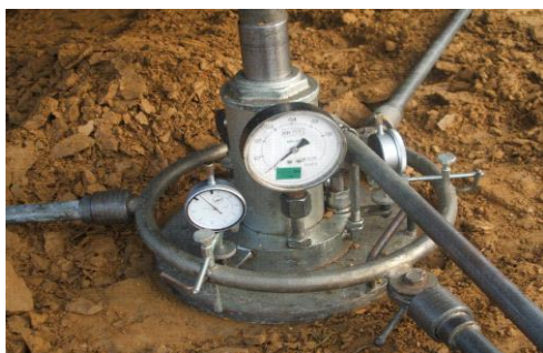
Figure 4. Static load plate
