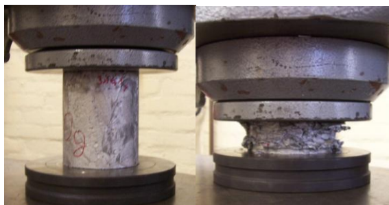
Figure 5 – Compression of aluminium foam sample
